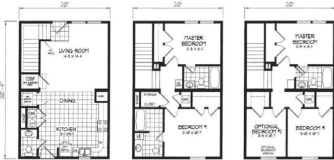
First Floor 600 Sq Ft Second Floor 600 Sq Ft 2 Bedroom Option Second Floor 600 Sq Ft 3 Bedroom Option
